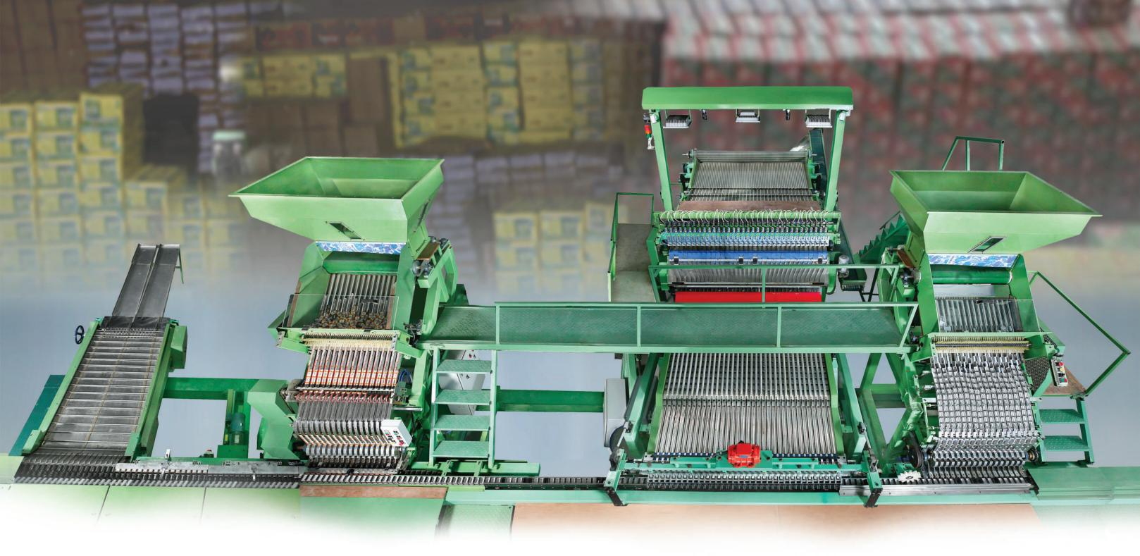
2016 was the year when we launched the world's first matchstick counting system, that revolutionised the way matchsticks are filled. In match industries maintaining the right stick count is essential to pass quality checks, boost the brand value and to maximise savings.
